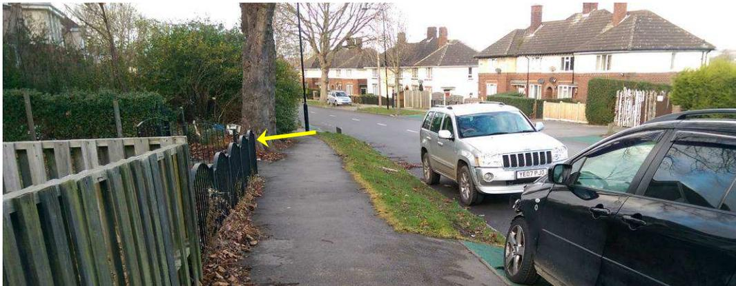
It will not be possible to construct the paved strip as indicated due to the severe gradient. In order to provide passenger access between the footway and bus-stop, significant civils works will be required. There will be a need for the provision of ramps and steps, as a minimum.
